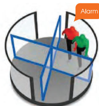
Door stops; Alarm activated
