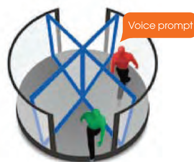
Door locks and then reverses to let unauthorized person go out
